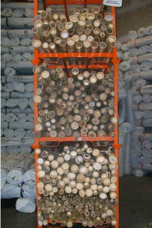
The tree structure is made of various diameter bamboo poles. Bamboo was chosen as the main building material because it's our intention to use green building materials whenever possible. It is a renewable resource that is lightweight and has the strength of steel. A large supply suitable for this project has been located at a local wholesaler's warehouse (<http://www.calibamboo.com>).
