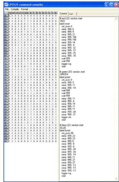
This first phase of software development creates the core technology for communication over the I2C bus to the LED boards. Next the artistic controls that create colors and patterns of light in each of the leaves will be developed.
