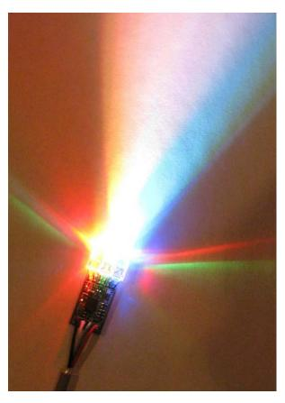
The custom LED board is capable of producing bright light of any color. A specialized control chip powers the individual red, green and blue LEDs, and is able to capable of producing very rapid and complex changes in the color of the light. Commands to the chip are sent over an I2C bus.
